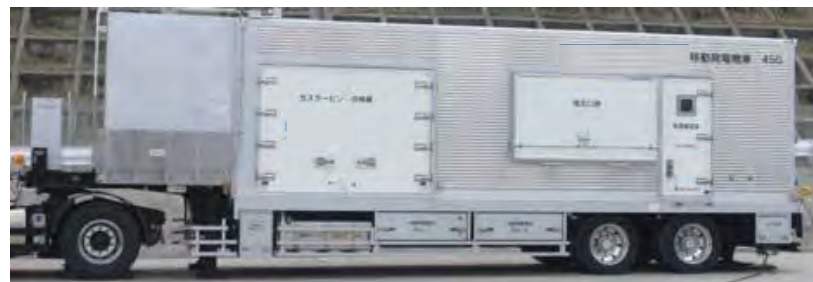
Alternative onsite AC power (Power Vehicle)
